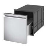
Self-contained, NSF certified, single-drawer in insulated cabinet. Single 304-stainless steel insulated drawer face mounted to full-size 8"depth hotel pan with 304-stainless steel tracks and acetal resin rollers. Drawer face measuring 12.75" x 16.25" has replaceable magnetic gasket providing a hermetic watertight seal. An insulated external jacket made from high-strength composite allows easy installation to indoor and outdoor kitchen cabinet installations.
