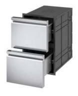
Self-contained, NSF certified, double-drawer in insulated cabinet. Double 304-stainless steel insulated drawers each mounted to full-size 8"depth hotel pan with 304-stainless steel tracks and acetal resin rollers. Overall double drawer face measuring 25.74" x 16.25", each drawer with replaceable magnetic gasket provides a hermetic watertight seal. An insulated external jacket made from high-strength composite allows easy installation to indoor and outdoor kitchen cabinet installations.
