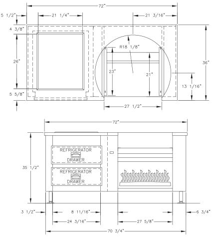
Note: gas and electric connectors are located on the bottom rear of the cabinet (cook surface side), 11.5" from the side. Connectors can be relocated on request.
